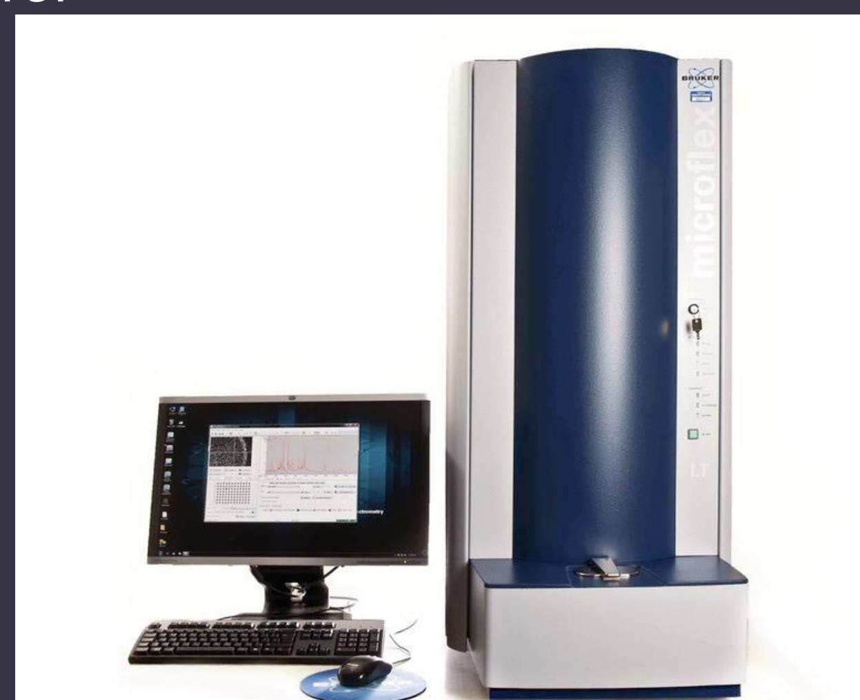
Figure 3. Bruker MALDI-TOF that was used for creation and validation of a database.
