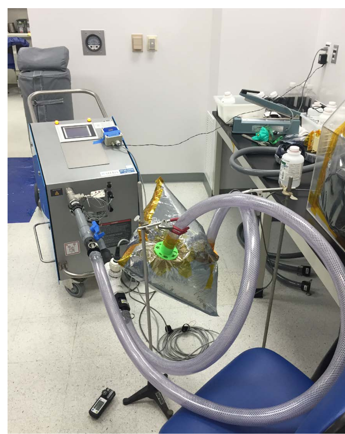
Fig 2. The enclosure attached to the VHP 1000ARD Biodecontamination unit
