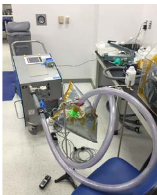
Fig 1. The enclosure attached to the VHP 1000ARD Biodecontamination unit
