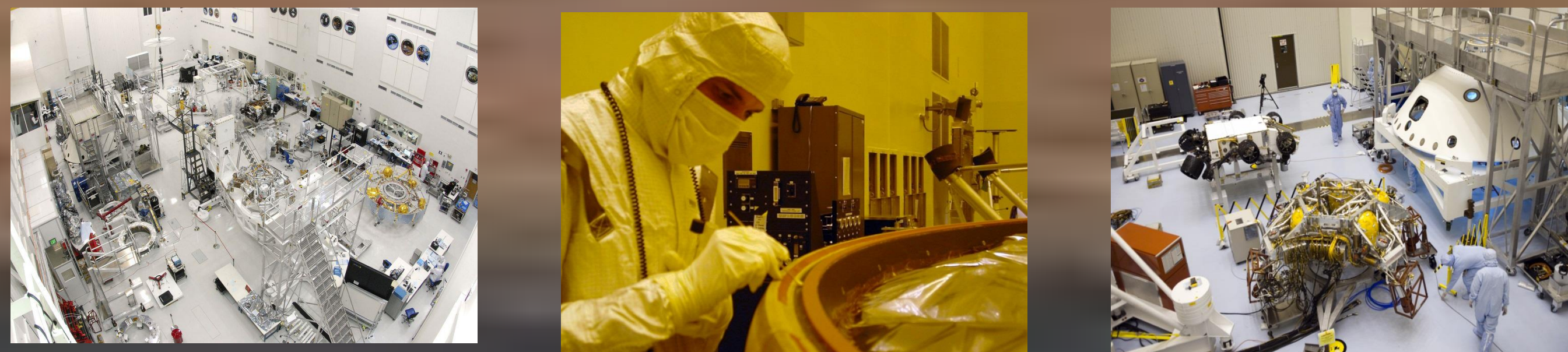
Cleanrooms at JPL (left) and Kennedy Space center (right) are used to assemble spacecraft. The center image depicts a swab sampling on a spacecraft part. Gloves and special clean room garments are required.
